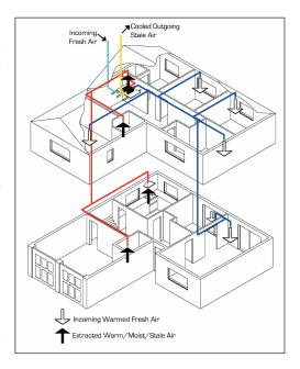
The system is designed to run continuously and should NOT be switched off except for maintenance or filter replacement. It is important to follow the advice in this user manual and correctly install and maintain the system to ensure a healthy and comfortable indoor environment.
